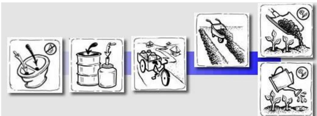
*Example of a sanitation chain with a diversion toilet, separate storage for excreta and urine, transport of tanks, composting and re-use of manure and urine (source: [www.akvo.org](http://www.akvo.org)).*
